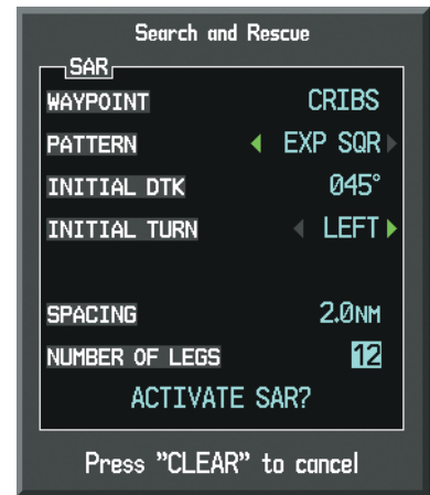
Pressing the ENT Key with the 'ACTIVATE SAR?' Field Highlighted Activates the Flight Plan
